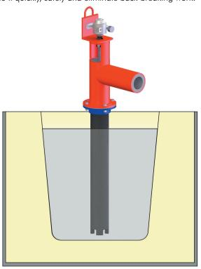
The Speed Demon is perfect for emptying filter or degassing boxes between alloy changes. It can also be used for emptying furnaces when repairs are required. Let the Speed Demon reduce your down time!
